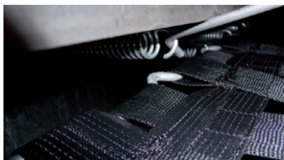
Hinging or unhinging the steel springs with the mounting tool
